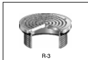
5" (125) round heavy duty stainless steel cleanout cover/plug with o-ring gasket
